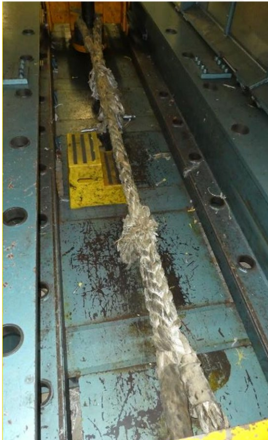
Before Pull to Breaking Force
