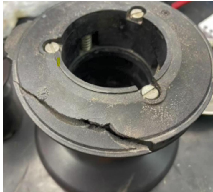
Pic 1: Winch: Broken upper Jaw
