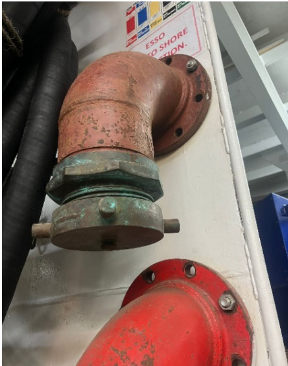
2 x 8" manifolds to connect to 2 x risers on main deck, in turn connected to 2 x 6" hoses from the terminal
