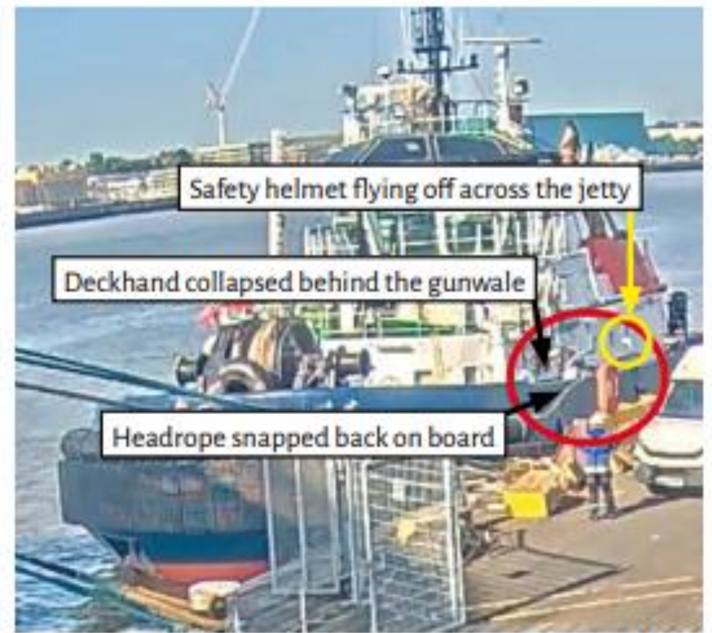
Figure 2: The headrope having snapped back and sent the deckhand's safety helmet flying
