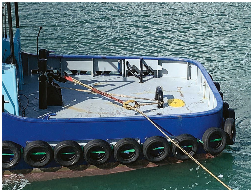
Figure 4(b). Vessel with a gog rope rigged
