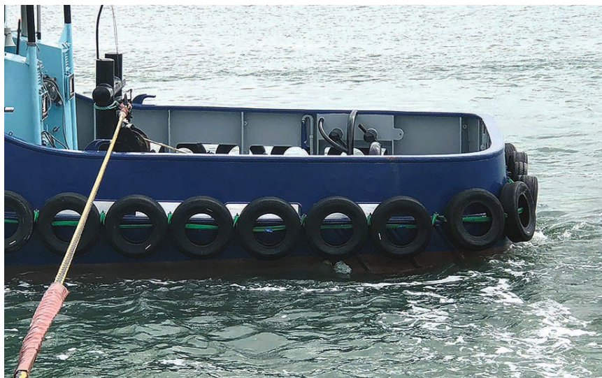
Figure 4(a). Vessel without a gog rope
